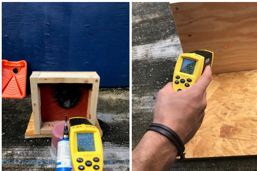
Figure 21. Fire testing a 18"x18" wooden test coupon after applying IC to 1/8" thickness using a slow pour method.
